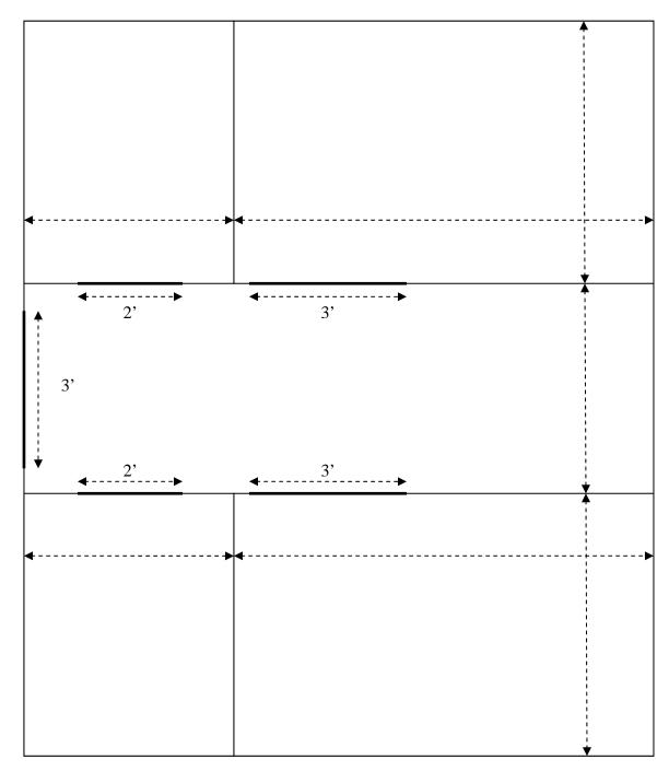
Figure 1. Mount Graham red squirrel soft-release enclosure design.
